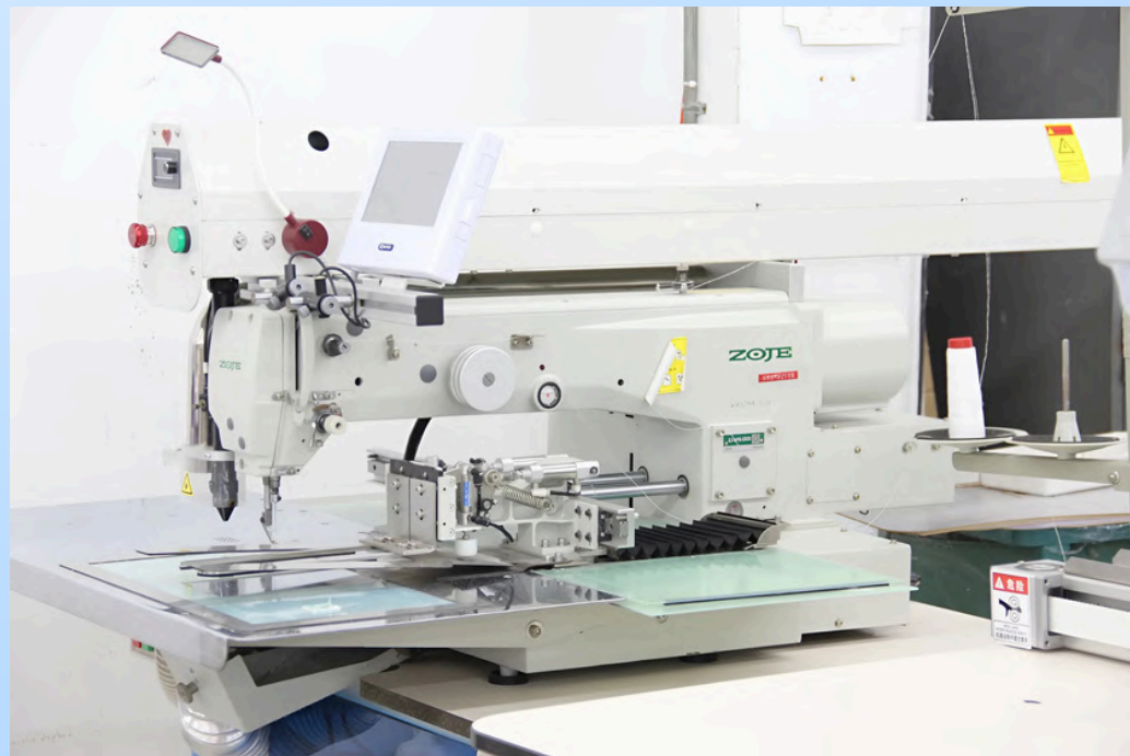
High-quality stitching of baby garments using industrial sewing machines
